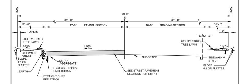
A MINIMUM 7FT WIDE PEDESTRIAN ACCESS ROUTE (PAR) SHALL BE PROVIDED BETWEEN OPPOSING RAMPS AND SHALL HAVE A CROSS-SLOPE (THE LONGITUDINAL STREET SLOPE) NO GREATER THAN 1.56%.
